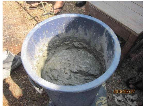
1.1-4 Bad mixing of APT (not available for testing)
