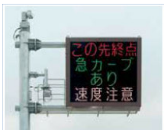
Figure A typical 4 row VMS board installed in Japan.
