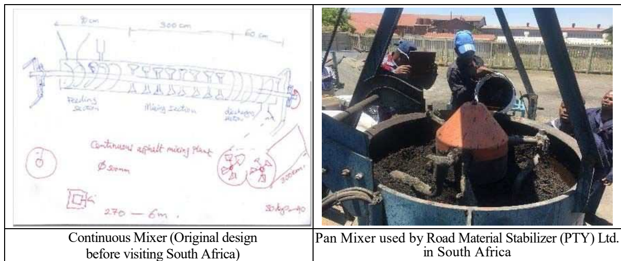
Figure 3: Comparison between the original design (Continuous Mixer) and Pan Mixer
