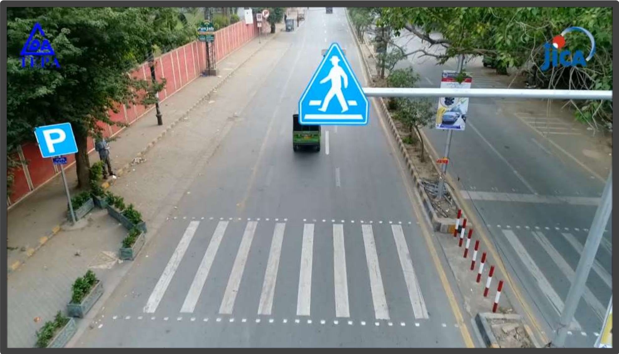
Non Signalized Crosswalk
