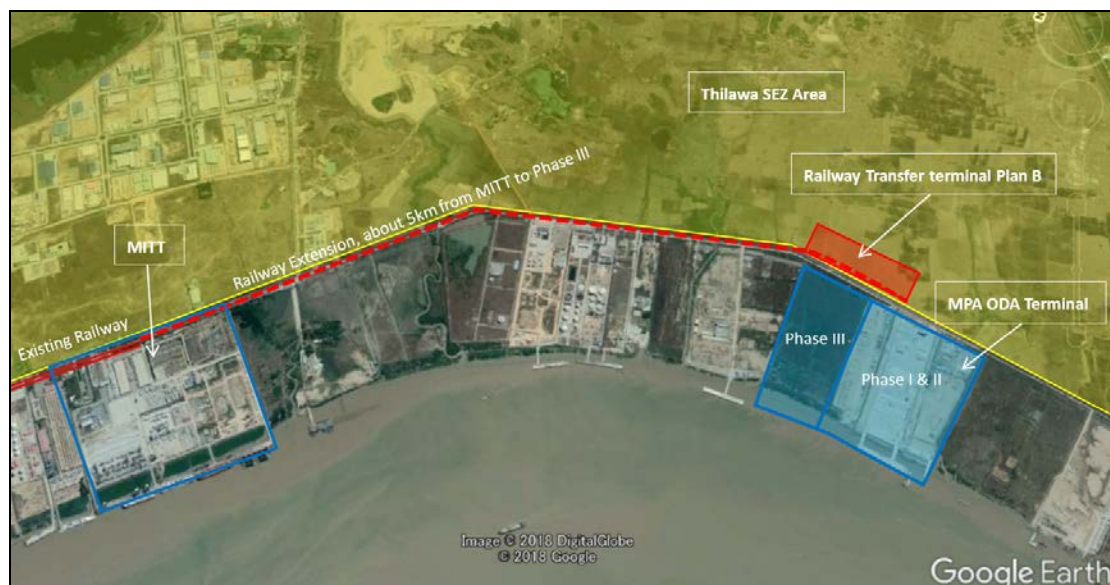
Figure 2.3.16 Railway Development Plan B (located in SEZ area, common use with other cargo from SEZ and other terminals)
