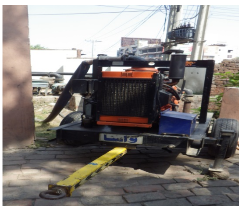
Potable Engine Pump
