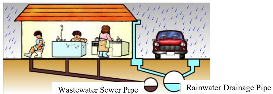
Figure 7.1-1 Image of Separate System
