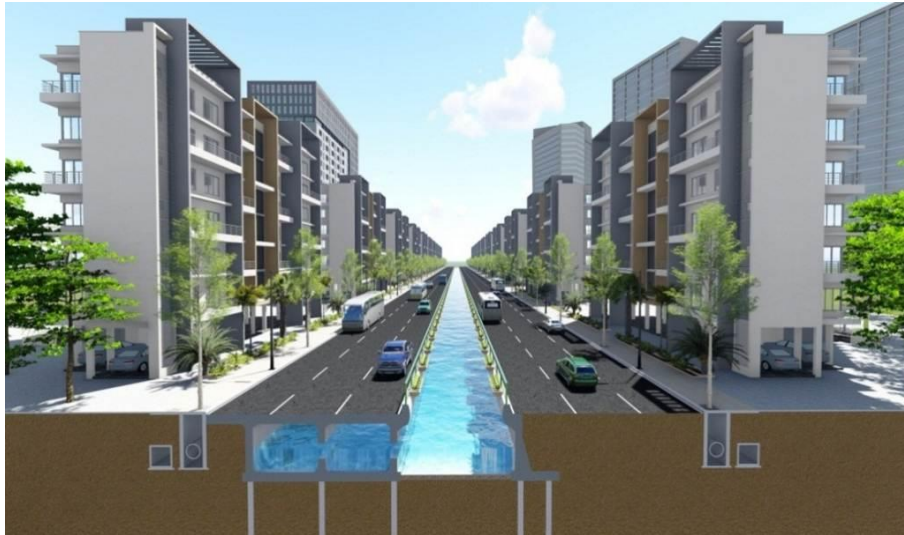
Figure 2.1-1 Image of Developed BOX Culverts and Open Ditch
