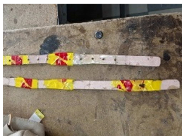
Photo 6 : Patterns used by the company. Could not be used due to severe damage.
