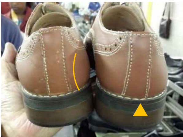
Photo 10: Soles not attached properly. Left: curve Right: Not center
