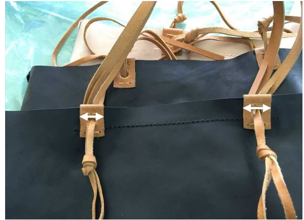
Photo 8: Inspection before shipping the first sample. The difference in leather piece's size on the right and left handle attachments (Dec. 2018)
