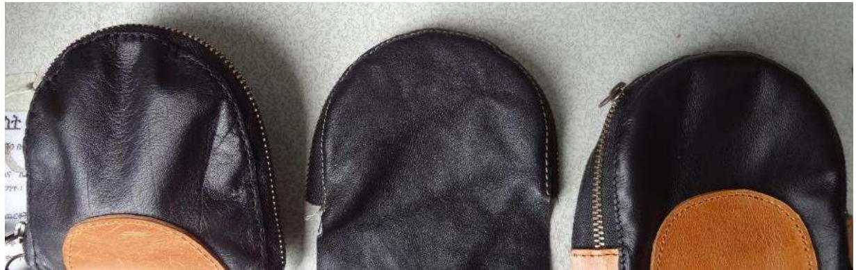
Photo 9 : Improvements through guidance on gluing and sewing: Left - before the guidance was given; Middle – expert sample; Right - after the guidance was given
