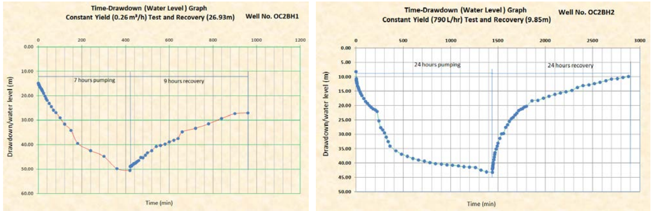
Figure 2: Constant rate and recovery OC2BH1 &OC2BH2
