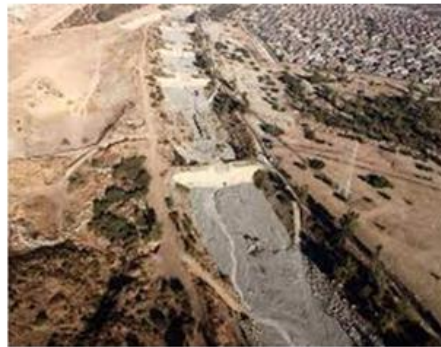
Decanting pools in the Macul ravine
