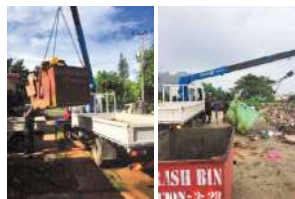
Garbage collection before the improvement. Approximately 350 steel containers are installed at Kolonia Town. The containers with full of garbage are loaded onto a flatbed truck with a crane, and the garbage is discharged at the disposal site.
