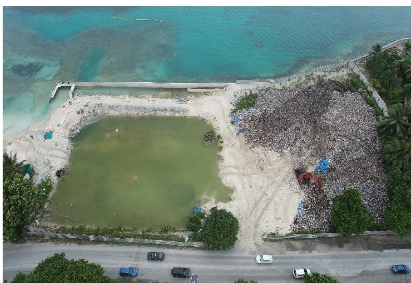
Figure 2: showing Cell 1 at the right, being filled, and Cell 2 at the left, under construction
