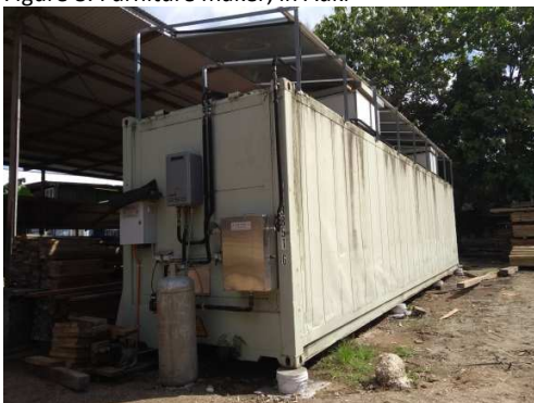
Figure 10: Timber kiln, in Honiara
