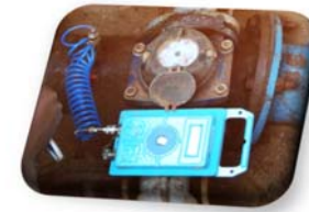
Figure 37 Example of Water pressure data loggers
