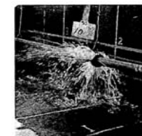
Dia.50mm Falling out of the flange portion (1/2 Full) Water pressure:2.0 kg/cm 2 , W/Leakage 10 m 3 /hrs. Water pressure: 2.5 kg/cm 2 , W/Leakage 11.2 m 3 /hrs Water pressure: 3.0 kg/cm 2 , W/Leakage 12.2 m 3 /hrs
