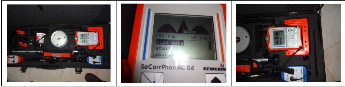
Figure-9 Overview of Leak noise correlator
