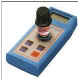
Residual chlorine analyzer
