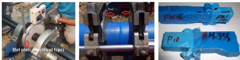
Figure-49 Topical Butt Fusion Joint
