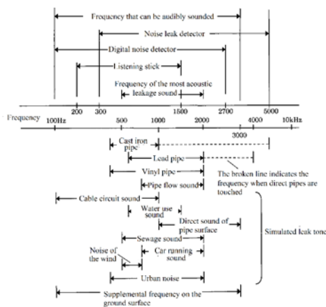
Figure 4: Range of hearing of leakage detection, and frequency of leakage
