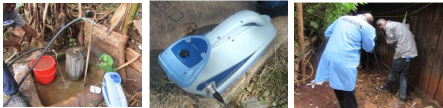
Figure-13 Overview of Vibration-wave water detector
