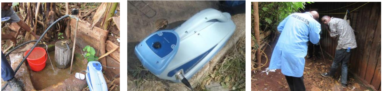
Figure-13 Overview of Vibration-wave water detector
