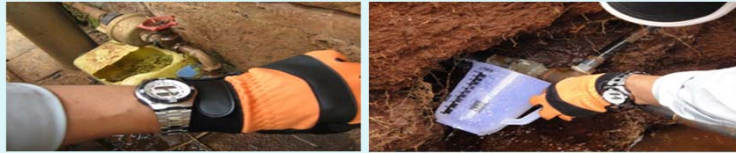
Direct measurement of leakage volume
