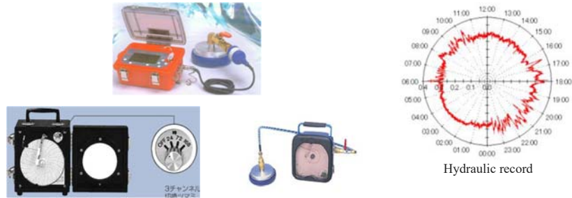
Figure 36 Example of Self-recording water pressure gauges
