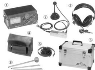
Figure-8 Overview of Road surface digital noise leak detector
