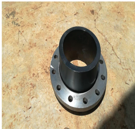
Figure 2.34: Stub end joint (Connects flanged steel pipe and PE pipe)
