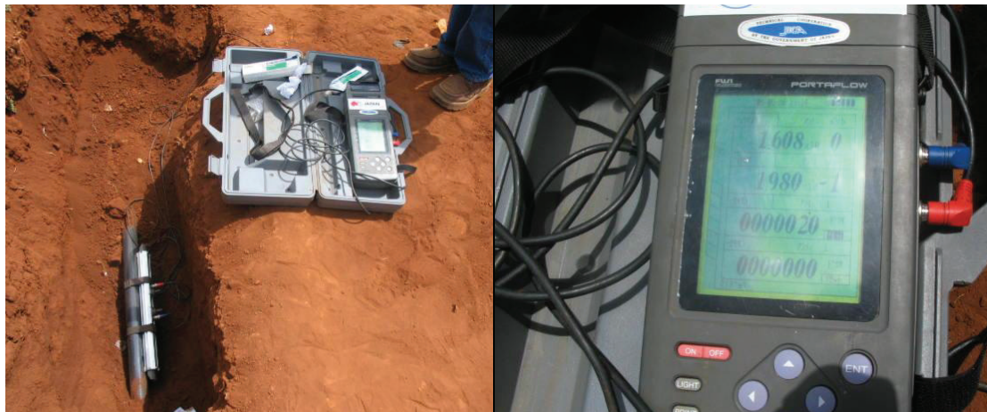
Figure 5.30: Flow Measurement Using UFM
