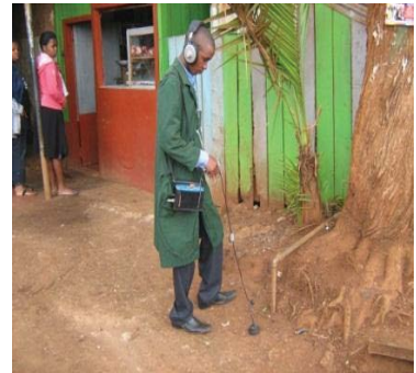
Figure 9.19: Leak detection using electronic leak detector
