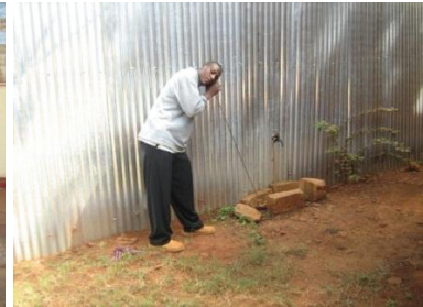
Figure 5.3: Leak detection using Listening Stick
