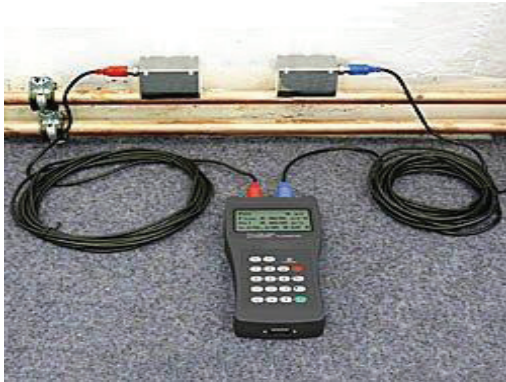
Figure 5.9: UFM mounted on pipe
