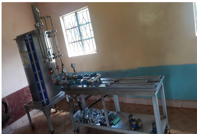
Figure 8.5: Water Meter Test Bench (EMBU WSP procured model)
