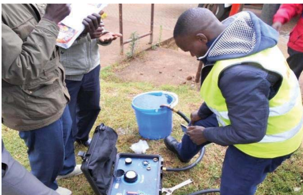
Figure 13.6: Meter Accuracy Test on Site Using Bucket and Meter Tester
