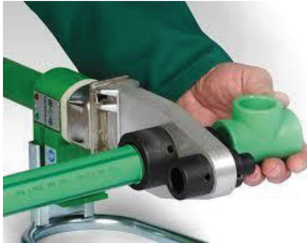
Figure 2.29: Heating PPR pipe & tee socket
