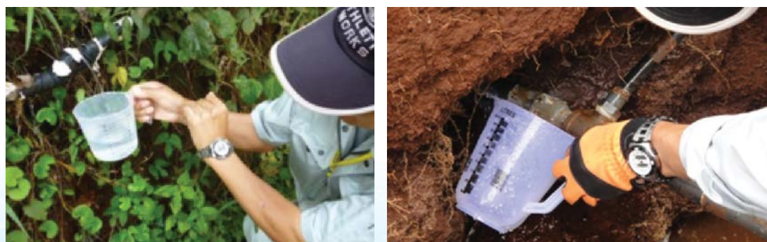
Figure 8.4: Measurement at Actual Leakage Point
