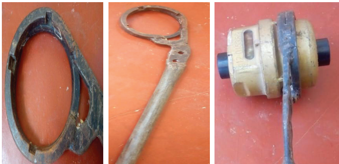
Figure 8.2: Custom-made spanner for Volumetric Type Meters
