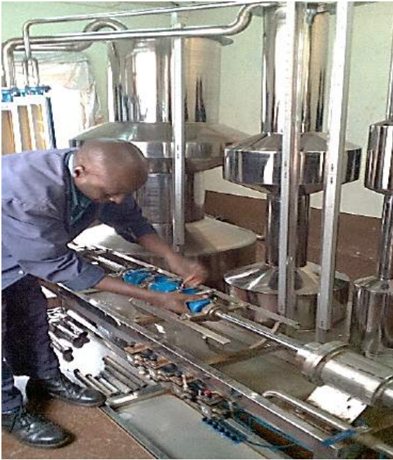
A technician testing the accuracy of consumer meters
