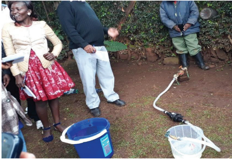
Figure 8.4: Testing a meter using calibrated bucket and a portable test meter
