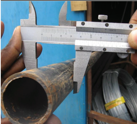
Figure 2.1: Measuring outside diameters of uPVC pipe with vernier caliper
