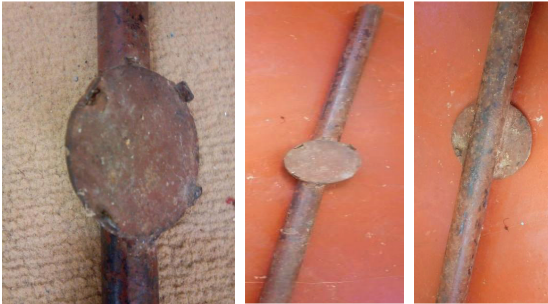
Figure 8.1: Custom-made spanner for Propeller Type Meters
