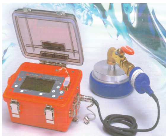
Figure 6.9: Self-recording water pressure measuring device model
