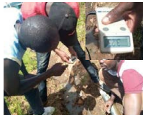
Figure 8.12: Using Ultrasonic Thickness Gauge to determine Pipe thickness
