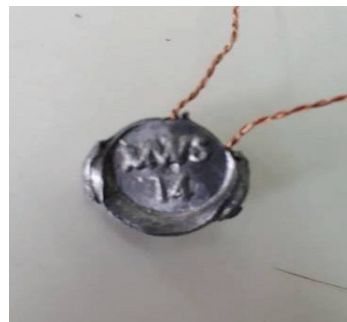
Figure 8.10: Sealing lead stamped by Pliers No. MWS14
