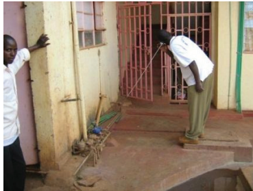
Figure 5.2: Leak detection using Listening Stick
