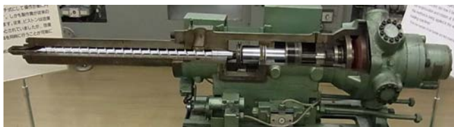
Cross section of inline screw structure
