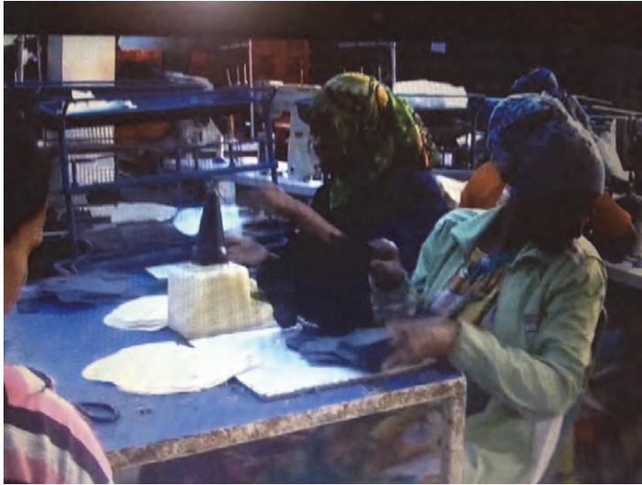
glue pasting lining with counter
