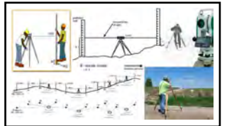
Figure 4-14 Ground level survey
