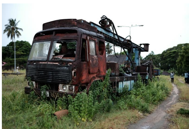
Photo 2.1 Ashok Leyland Rotary Type Drilling Rig
