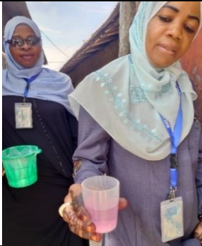
Photo 15: Pack test during meter reading survey 0.3 to 0.4mg/L of residual chlorine was detected by a pack test by the survey team during meter reading survey
