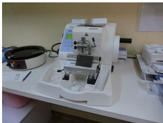
Electric microtome, good operation
