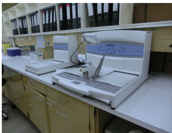
Embedding station (used for heating and cold treatment of embedded paraffin)
