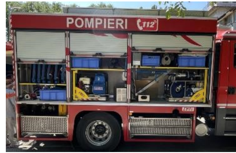
Photo 2-3 Lockers and aluminium shutters for storage on existing fire trucks
