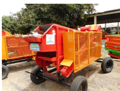
Brazilian threshers, threshing teeth are made of band steel with oscillating sheave
