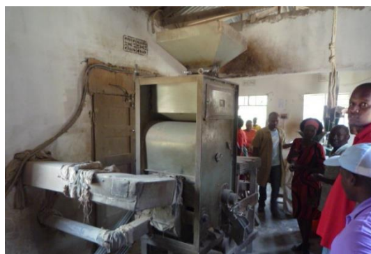
Photograph 5-7 One-pass type rice milling machine at a flour mill of the above Photo 5-6
