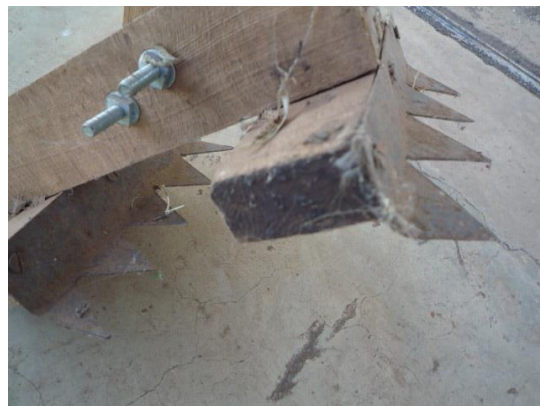
Serrated iron plates are used for scratching the surface of the paddy field and removing weeds, but the wood is thick, therefore there is hand-pushing resistance.
