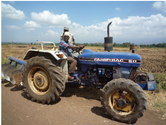
The field was plowed by a 3-disc plow. After this, the field was flooded and puddling was carried out. In this way, the plowing of straw and puddling (pulverizing soil) will be better than direct puddling work.
