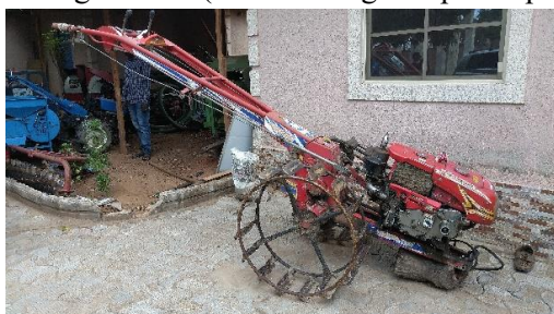
Photograph 4-7 A Pakistan-made power tiller and a towing-type puddling rotor
