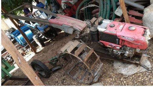
Photograph 4-8 Thailand Kubota power tiller (left) and Yanmar (Indonesia) thresher (right) (The engine of the thresher is a Chinese hopper-type 14 hp)
