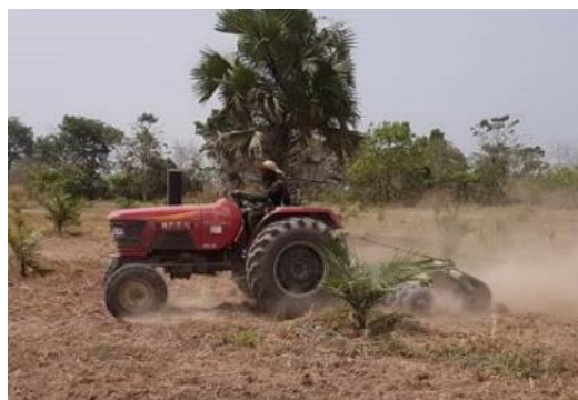
Photograph 4-1 Plowing with a disc plow (left) and harrowing with a disc harrow (right)
