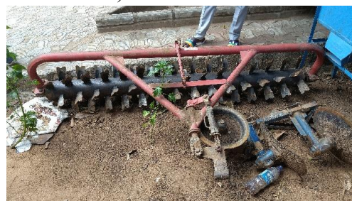
Photograph 4-7 A Pakistan-made power tiller and a towing-type puddling rotor
