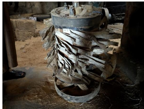
Polishing device, which removes bran powder from the surface of white rice. It is installed under the machine.
