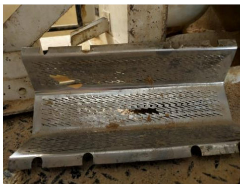
Photograph 4-15 Damaged screen of the rice whitening section
