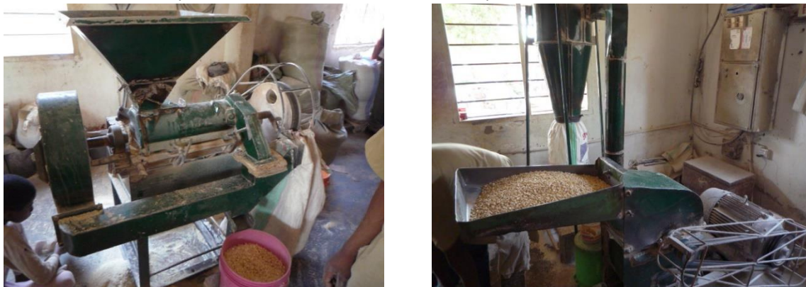
The Engelberg (left), and Hammer mill (right) are utilized not only for maize but also for millets, sorghum, and broken rice for use in a flour milling machine.
