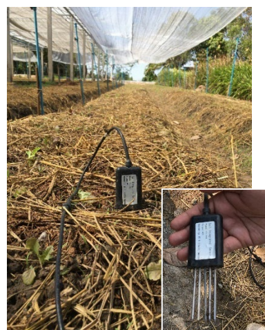
Soil sensor: by five pins, pH, NPK, soil moisture, soil temperature, and EC can be detected and recorded.
