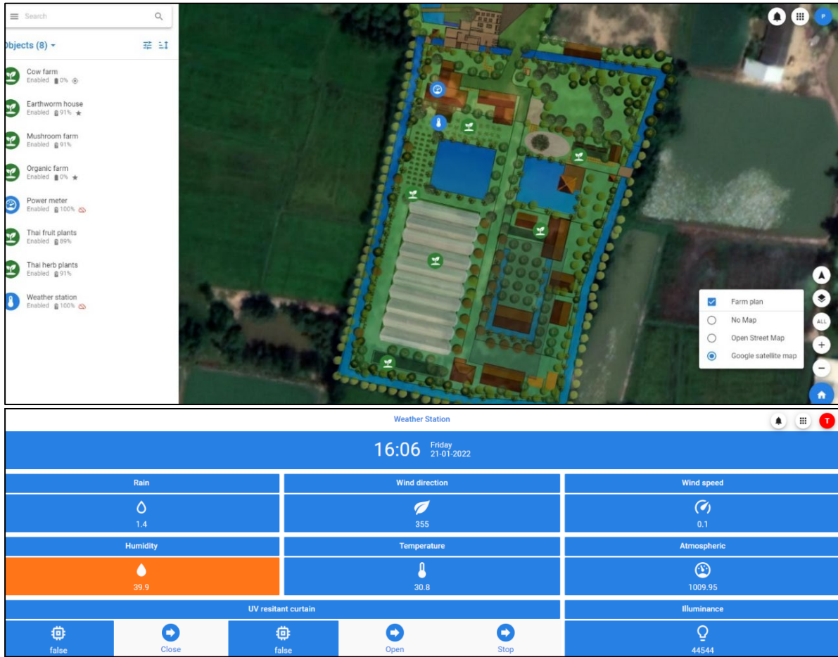
Figure 7.2.4 Weather Station Monitoring Screen (including operation mode of shading curtain)
