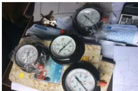
4 nos of Pressure Gauge received but not installed.
