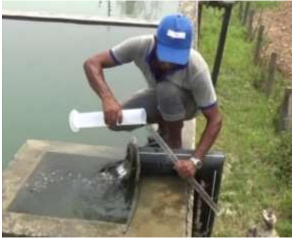
Photo 2.8 Measurement of Turbidity
