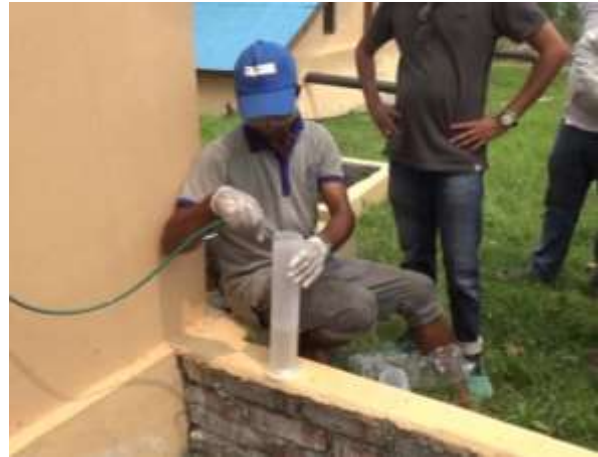
Photo-6. Weekly Inspection of Pump (Discharge Amount)
