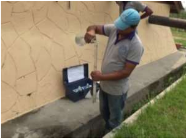
Photo 2.21 Measurement of Turbidity
