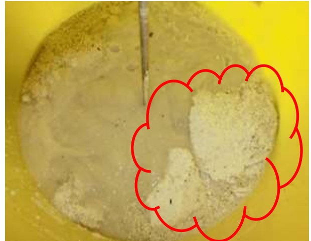
Photo-3. Adding Bleaching Powder (Left) and Appearance of Un-dissolved Lumps (Right)
