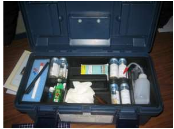
Figure 2.1 POTATEST (Wagtech, Left) and ENPHO Water Test Kit (Right)
