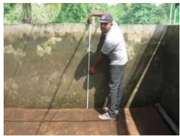
Photo 2.17 Measurement of Sand Layer Thickness
