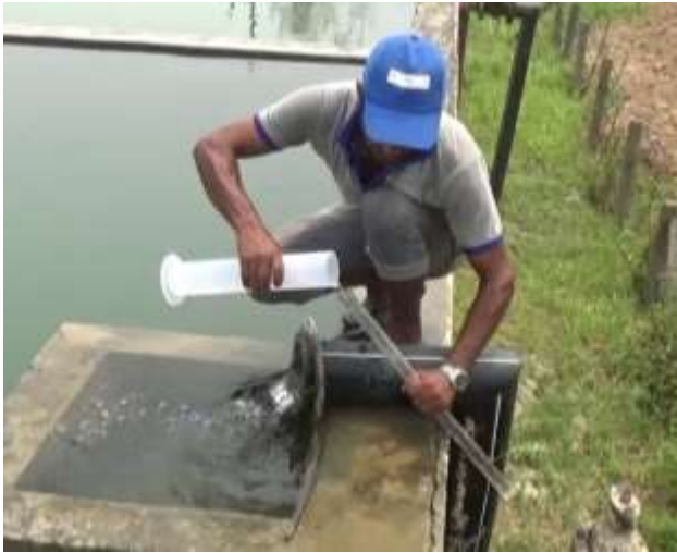
Photo-1. Measurement of Turbidity
