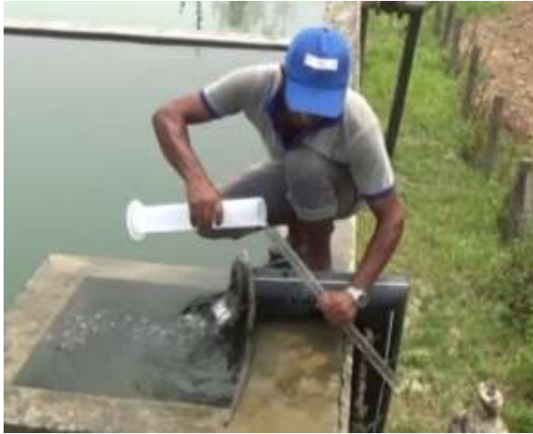
Photo 2.14 Measurement of Turbidity
