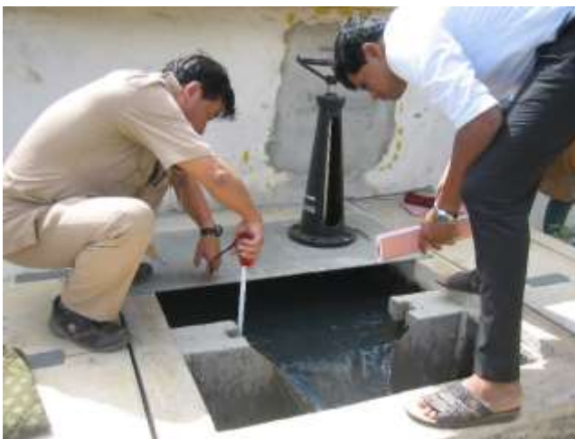
Photo-3. Measurement of Filtration Rate at V-notch
