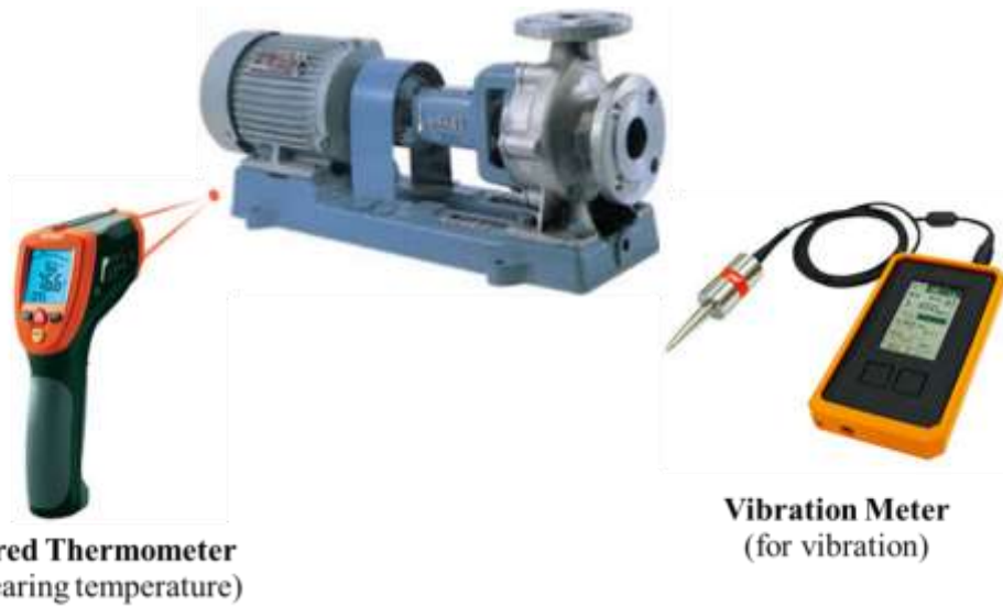
Figure 2.13 Measuring the Bearing Temperature and Vibration in Yearly Inspection
