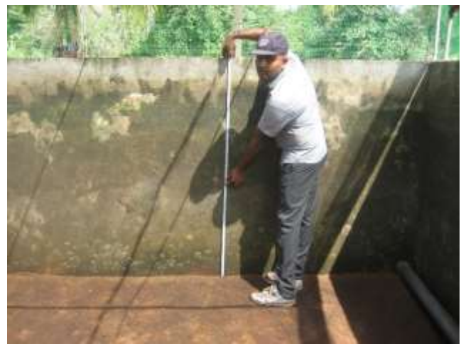
Photo-4. Measurement of Sand Layer Thickness
