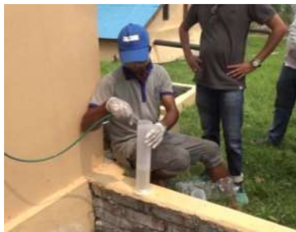
Photo 2.29 Weekly Inspection of Pump (Discharge Amount)
