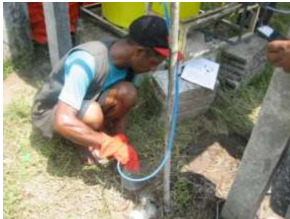
Figure 2.10 Checking the Actual Chlorine Dosing Amount by Using Measuring Cylinder
