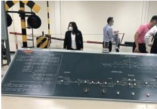
Photo. 2.4-28 Signal Control Panel and Rail Crossing Device
