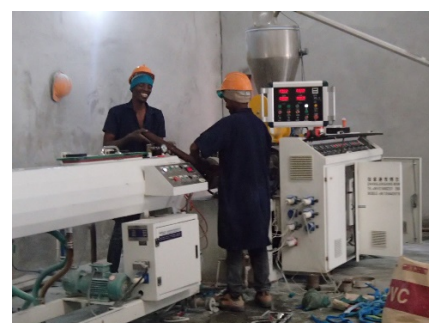
Company Visit at Mosh: Jeck Electrical: Newly purchased Vinyl pipe manufacturing machine. The owner said it is difficult to find technicians who can handle trouble.
