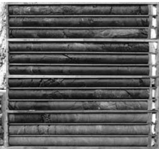
Core samples by hybrid drilling method
