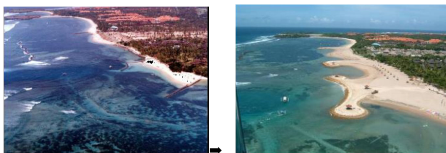
Figure 4-91 Aerial view of changes after sand nourishment, case of Sanur Beach, Bali
