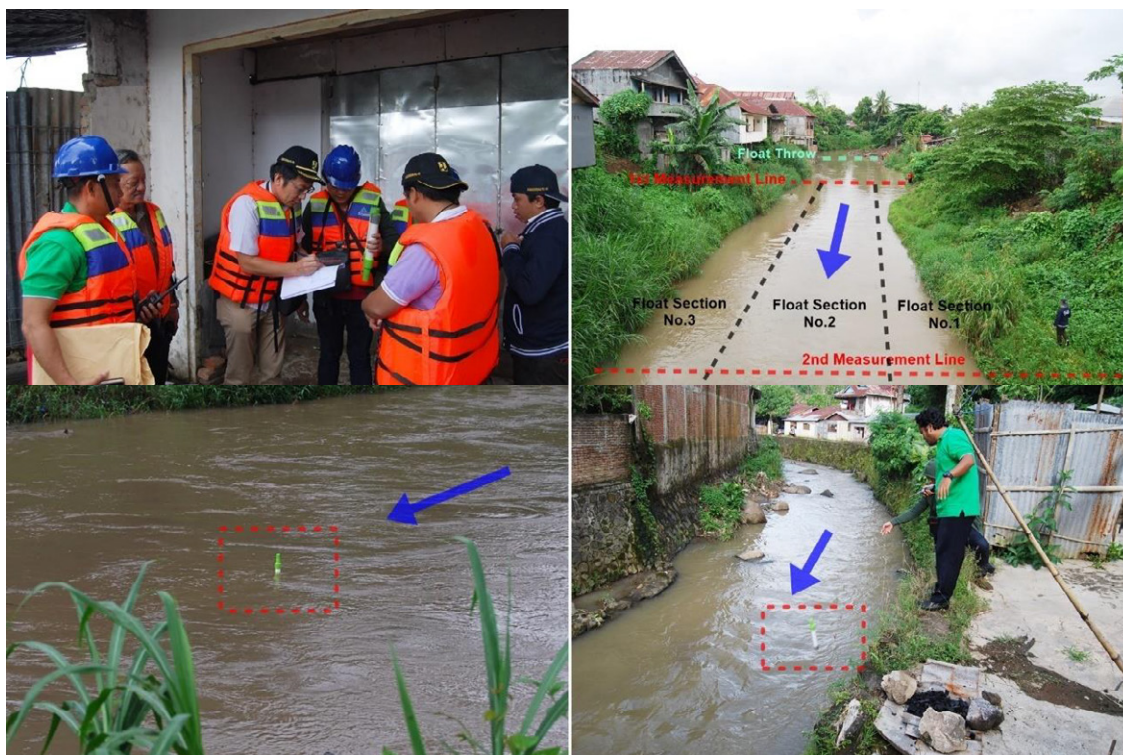
Photo 2.1.8 Site Practice of High Water Flow Measurement with BWS Sulawesi 1 (1/2)
