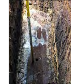
Core sample (S2) was taken from second compacted layer.
