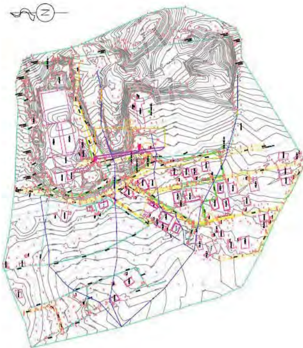
Figure 2-2 Identified surface water pathways
