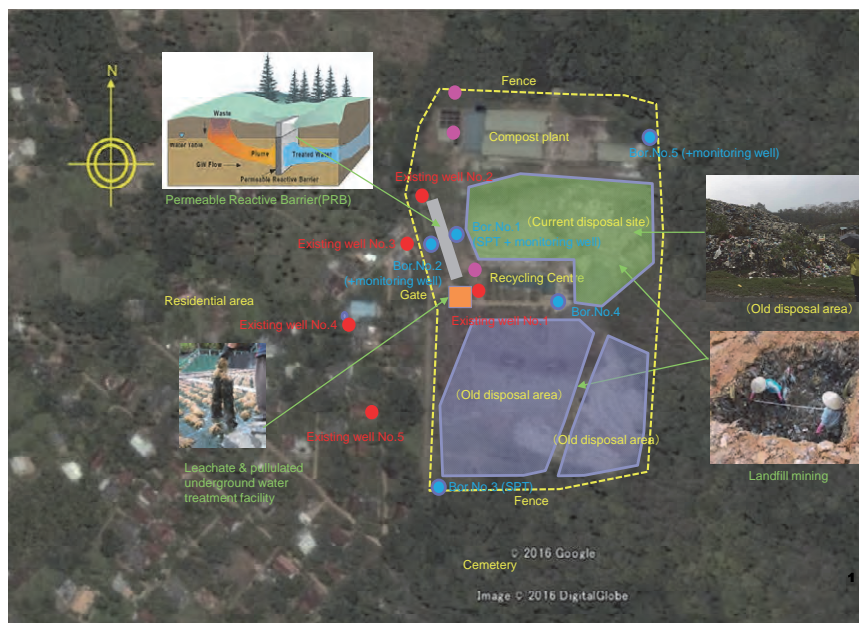
Figure 2-27: Sample points of water quality survey at Sundarapola disposal site in KMC
