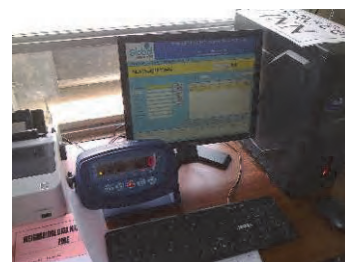
Weigh bridge data management system
