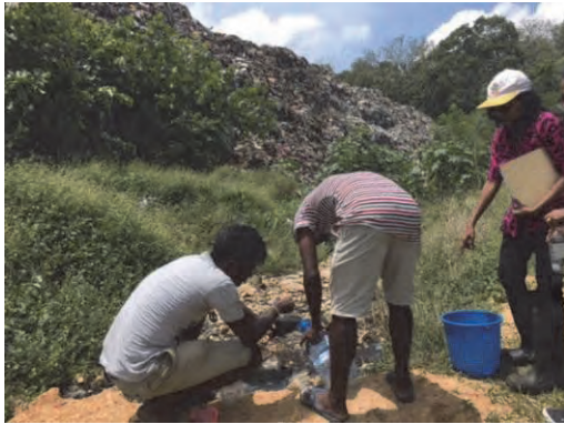
Leachate sampling at the disposal site in KMC
