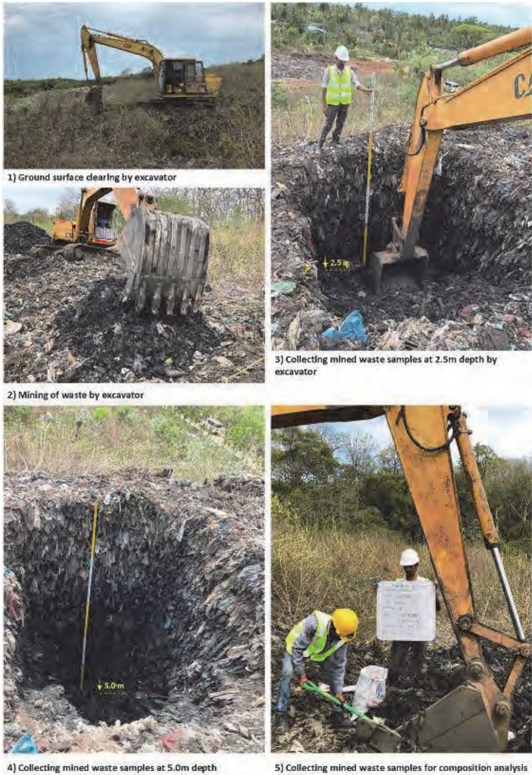
Figure 2-35: Mining of dumpsite and waste sampling procedure
