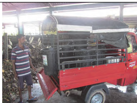
Collection of biodegradable waste by a three wheeler with installation of large bins
