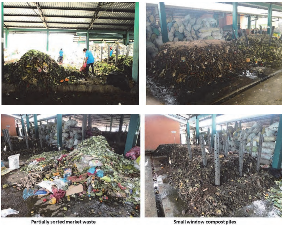
Figure 2-6: Windrow composting system in RMC
