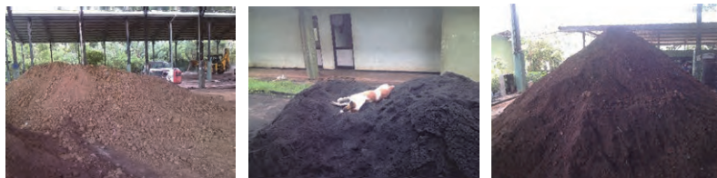
Bangadeniya Soil 12.5% : Biochar 12.5% : Brick particles 75.0%
