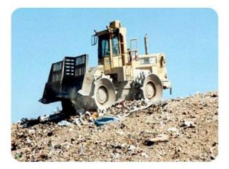
Figure 7.3.2 Compaction of the wastes at the landfill
