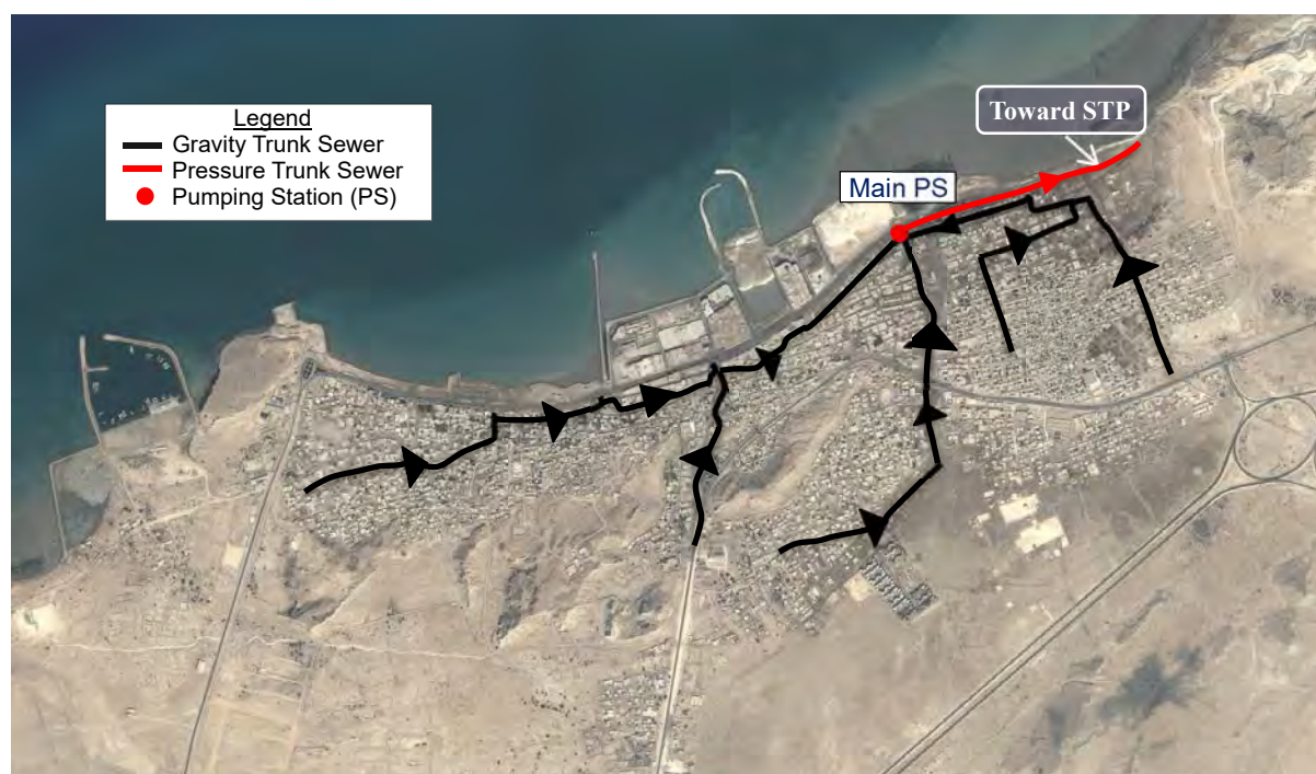
Figure 11.4.1 Trunk Sewer and Pumping Station Proposed in the Initial Stage Development
