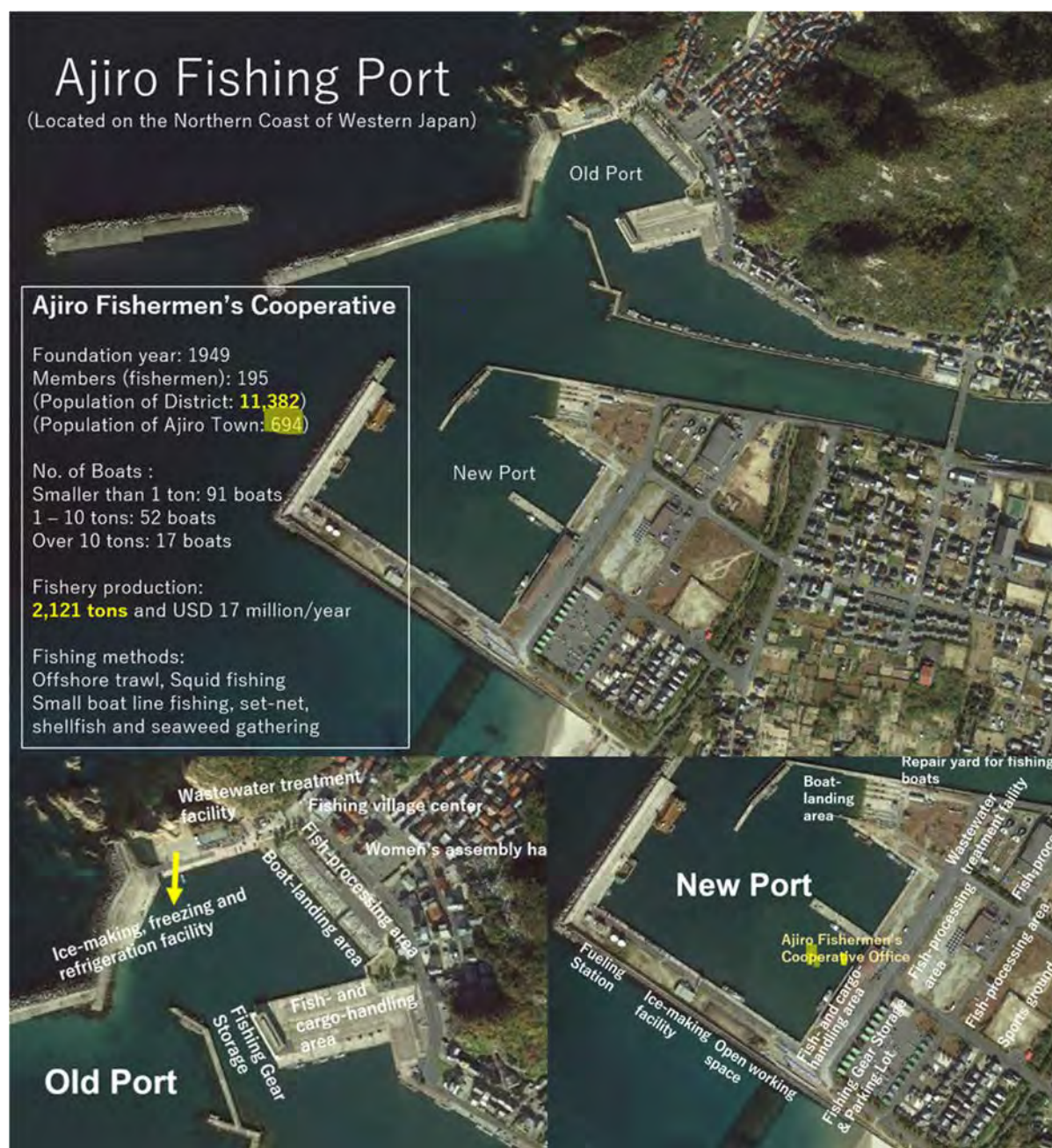
Figure 11.3.21 An Example of the Spatial Arrangement of Ice-making Facility, Refrigeration Facility, Fish- and Cargo-handling Area, etc. at a Fishing Port in Japan (Ajiro, Iwami, Tottori Prefecture)
