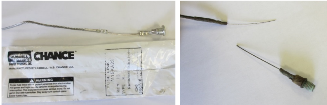
Figure 9-1-2.6 Example of an enclosed fuse installed on a PPUC power line (left, new product; right, after fusing)
