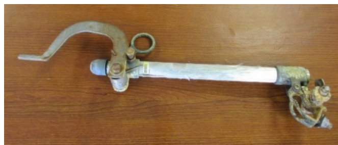
Figure 9-1-2.5 PC (primary cutout) enclosed fuse (installed on a power line with a fuse attached inside)
