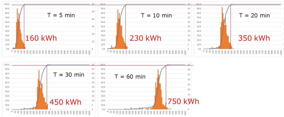
**Figure 5-2-2-9 Histograms of the battery capacity (kWh) for each moving average time (T)**
