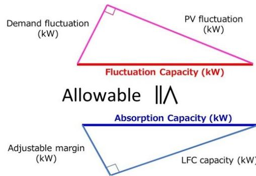
**Figure 5-2-2-2.1 Relationship between fluctuation and absorption sources in the algebraic method**
