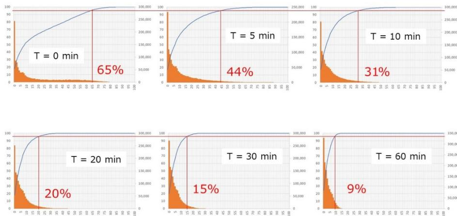
**Figure 5-2-2-2.6 Histograms of the fluctuation rate of the PV power station output for each moving average time (T)**
