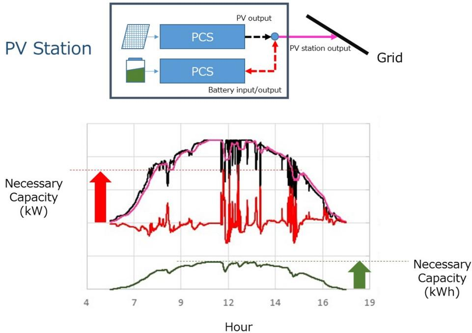
**Figure 5-2-2.7 Charge and discharge**
