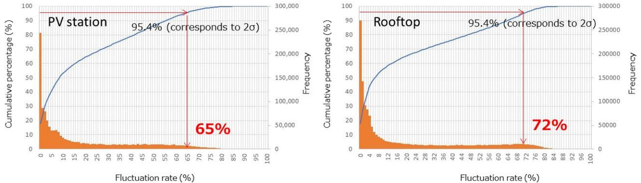
**Figure 5-2-2-2.3 Histogram of the output fluctuation ratio for PV systems**
