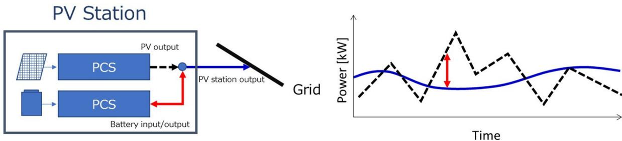
**Figure 5-2-2.4 Battery system model for suppressing the fluctuation of the PV power station output**
