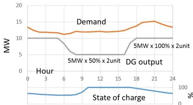
**Figure 5-2-2-1.12 Curves of demand, DEG output, and state of charge on the same day obtained by HomerPro**
