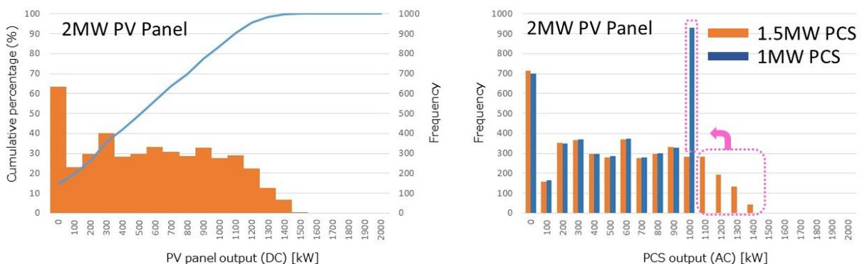
**Figure 5-2-2-1.2 Histogram for PV system output (left, PV panel output; right, PCS output)**
