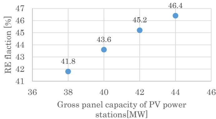
**Figure 5-2-2-1.9 Relationship between the panel capacity and RE ratio of PV power station**
