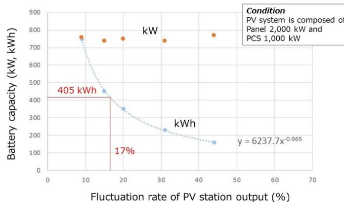
**Figure 5-2-2-2.10 Relationship between the fluctuation rate and battery capacity**
