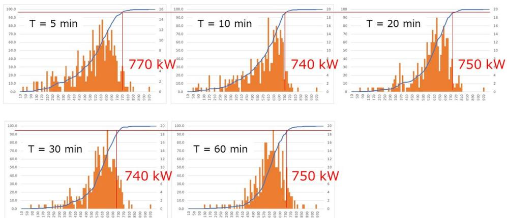
**Figure 5-2-2.8 Histograms of the battery capacity (kW) for each moving average time (T)**
