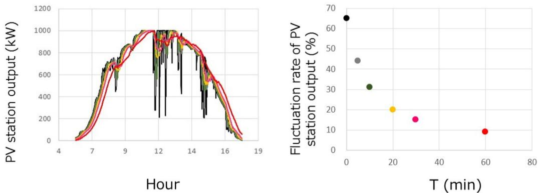
**Figure 5-2-2-2.5 Relationship between the moving average time (T), PV power station output, and the output fluctuation rate (left, PV power station output; right, fluctuation rate)**
