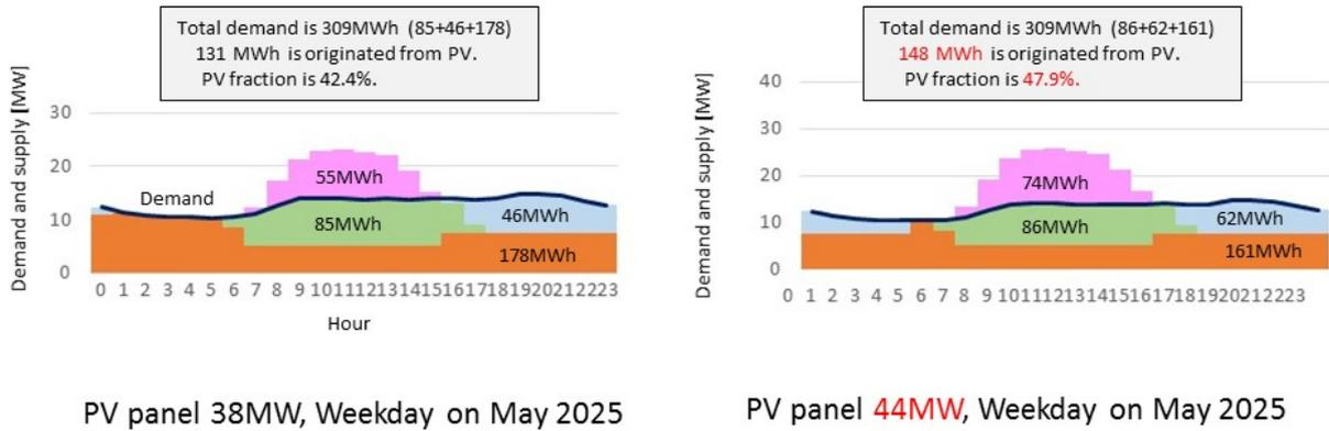
**Figure 5-2-2-1.8 Improvement of RE ratio by additional installation of PV**
