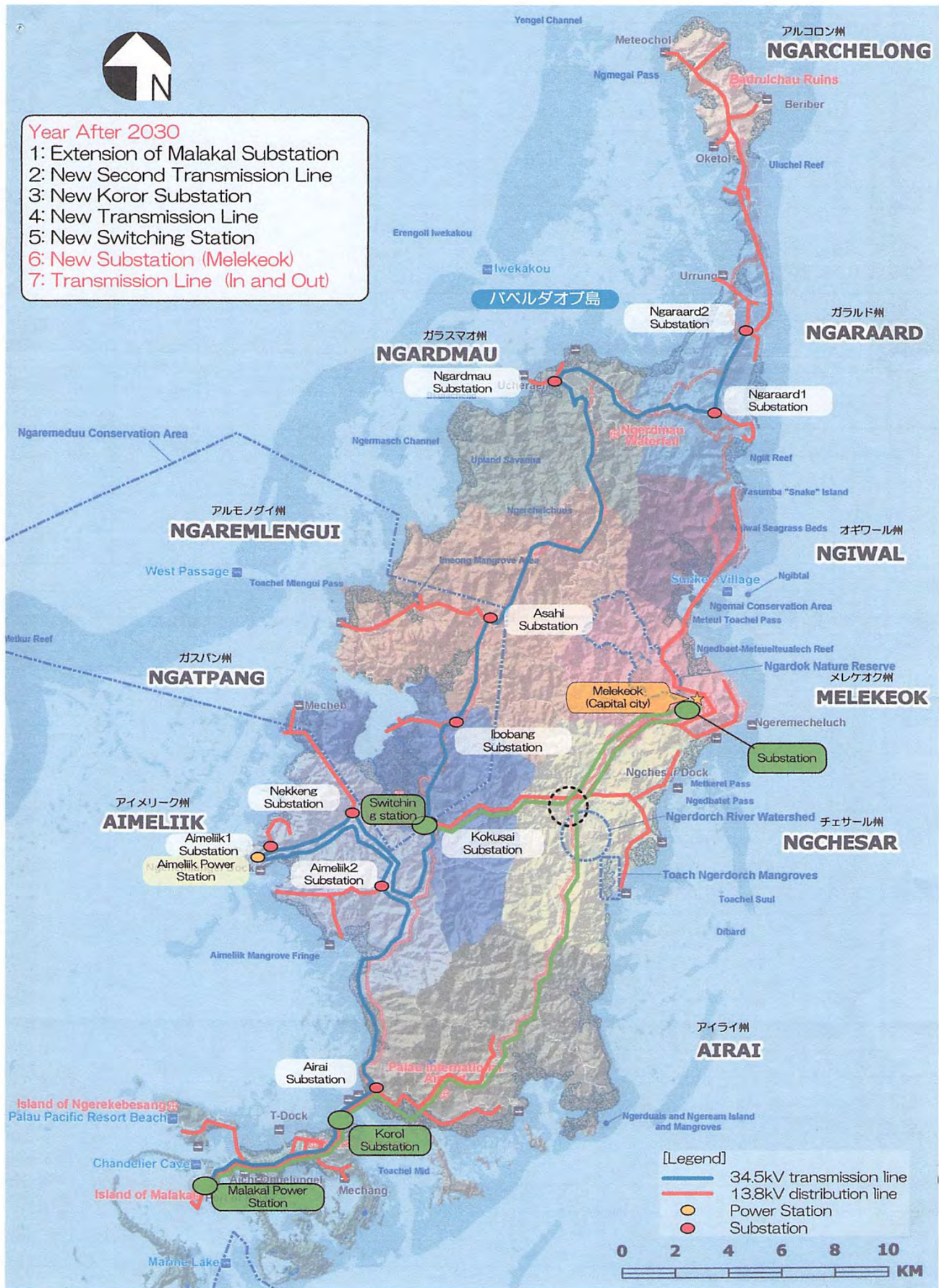
Appendix-4: Preliminary Location Map of Transmission Lines, Distribution Lines and Substations (After Year 2030)
