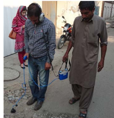
Leakage Survey by Leak Detector
