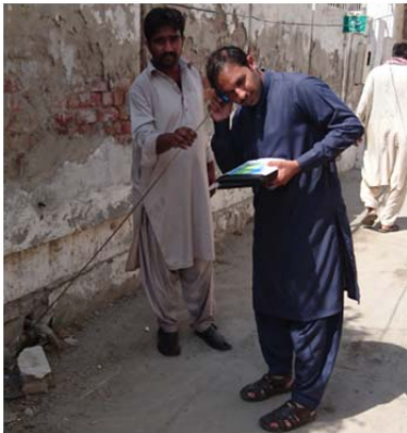
Leakage Survey by Acoustic Rod
