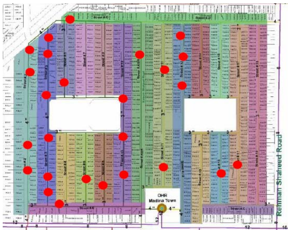
Figure 3.2.5 Locations of Leakage and Repair in Madina Town
