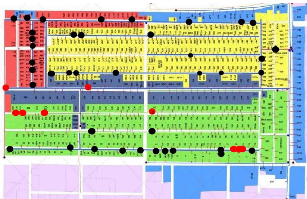
Figure 3.1.8 Locations of Leakage Survey in Sarfraz Colony Pilot Area
