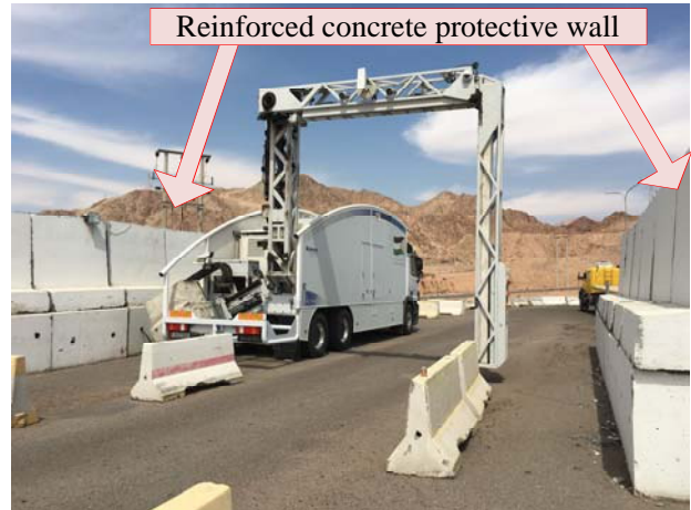
Photo 2-1 Reinforced concrete protective wall and X-ray inspection machine
