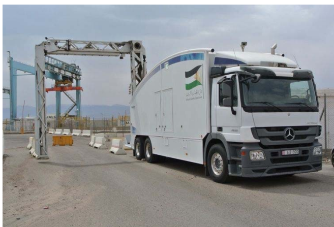
Mobile type X-ray inspection machine at ACT
