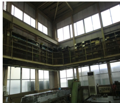
Utilizing the vertical space to store materials
