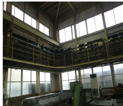
Utilizing the vertical space to store materials
