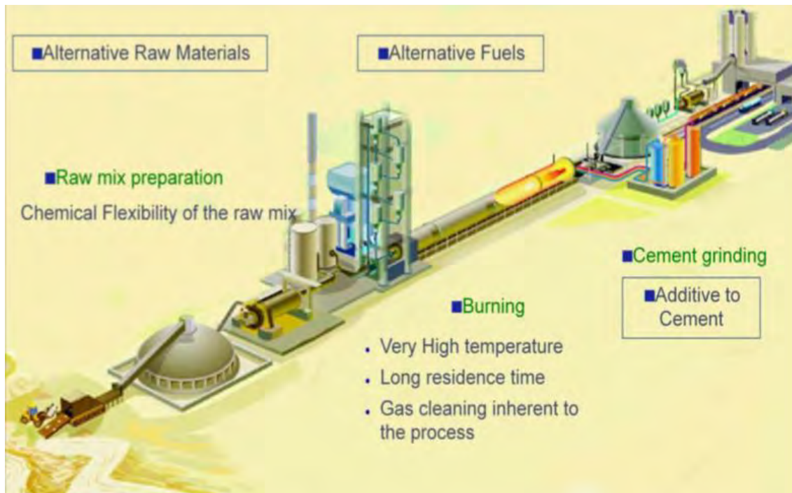
Figure 4.1-1: A Closed Cycle Process Without Residual or Waste/Byproduct
