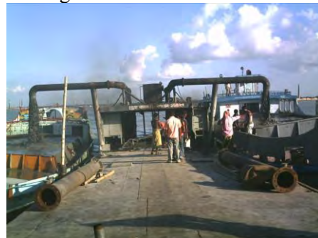
Dredging of fill material from the river bed at Meghna river by pumping up
