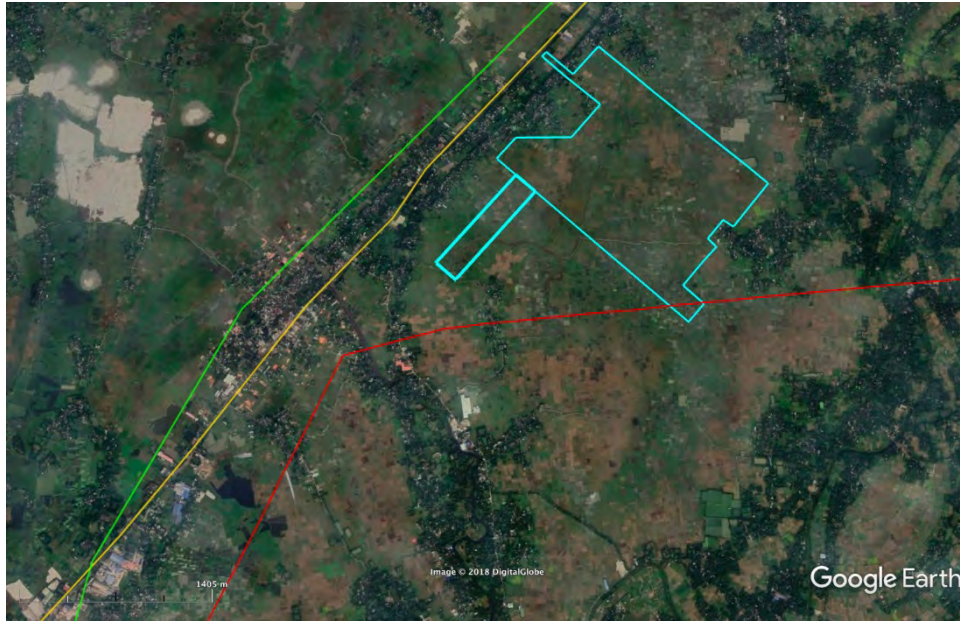
Figure-S 2.5-9: 132kV and 230kV transmission lines Green line: 132kV transmission line, Red line: 230kV transmission line, Yellow line: Dhaka-Sylhet National Highway N2, Blue line: proposed EZ boundary
