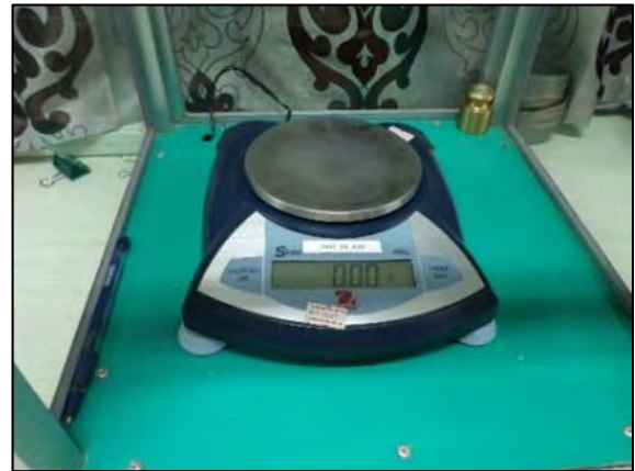
Photo - 1.7 Electrical Balance
