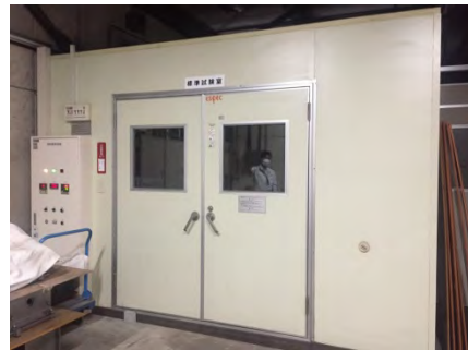
10) Material Testing Building (Standard Testing Room, Temp. 20°C, Humidity 80%)
