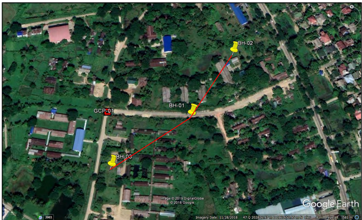
Figure - 3.7 Borehole Location and Soil Profile on Google Map
