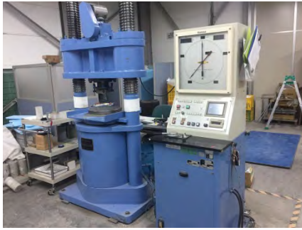
13) Material Testing Building (Universal Testing Machine (500kN))
