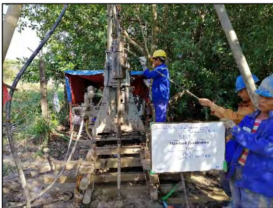
Photo - 3.5 View of Standard Penetration Test and SPT Sample
