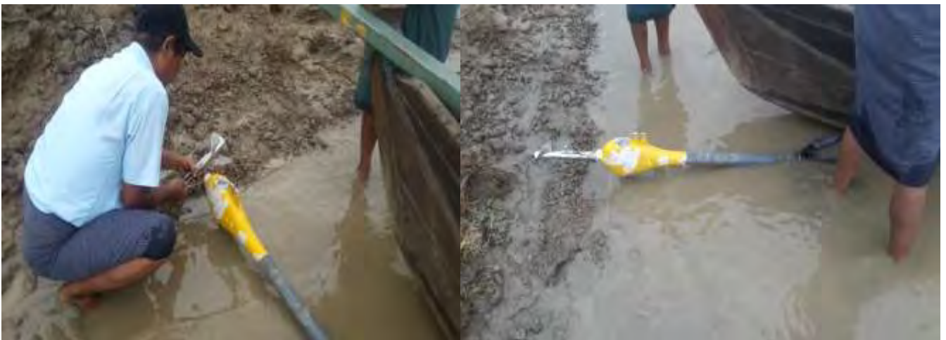
Figure 28 Equipment of Water Flow Velocity Measurement
