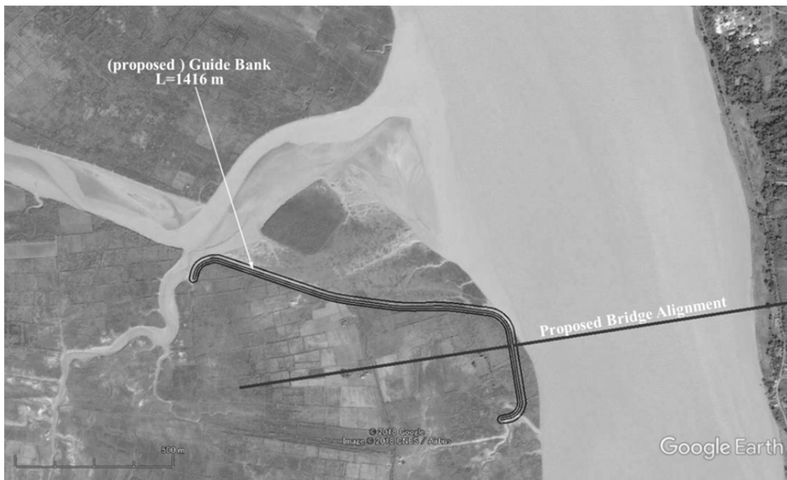
Figure S 7.3.1 Proposed Guide Bank at Right Bank
