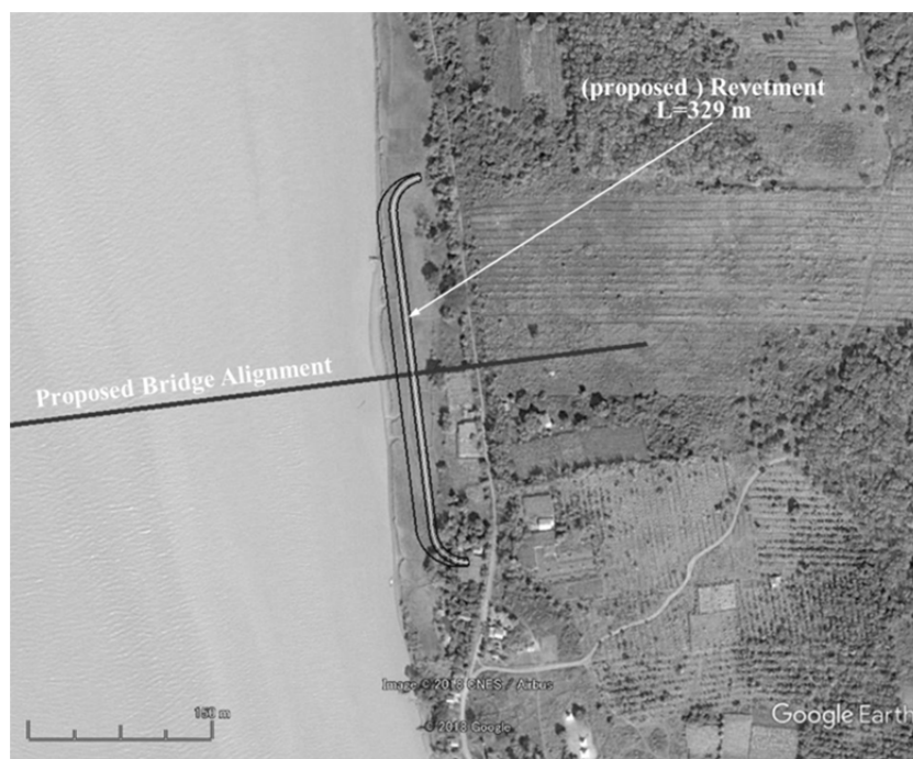
Figure S 7.3.3 Proposed Guide Bank at Left Bank
