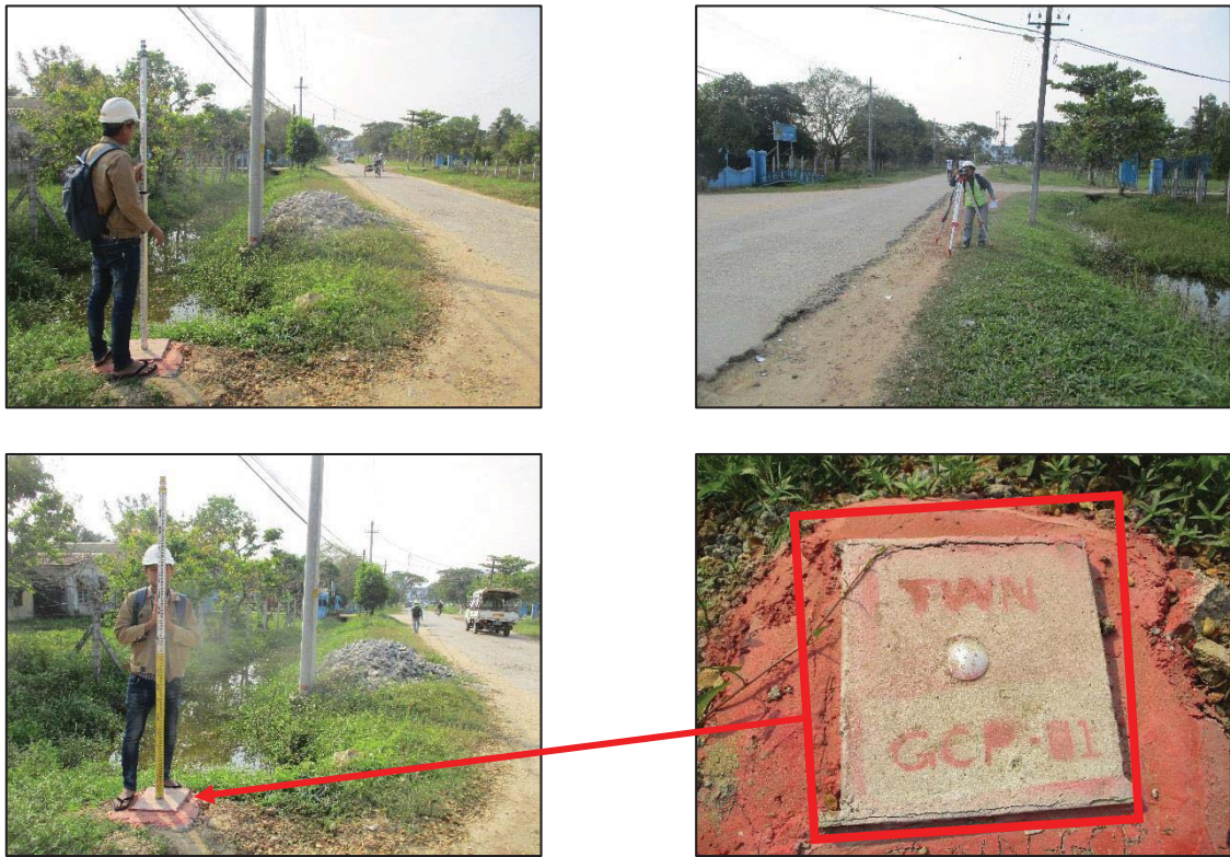
Photo - 3.1 Leveling Process and Control Point (GCP-01)
