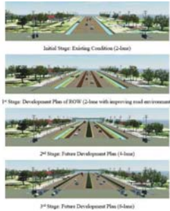
Figure 4.2 Construction Start from the middle of the ROW
