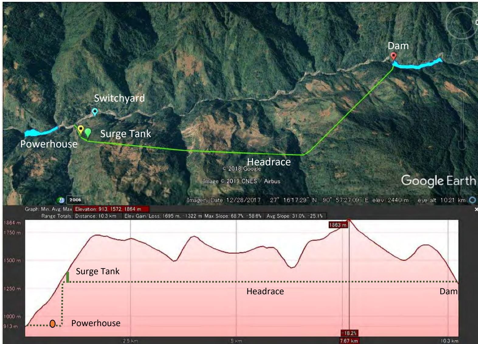
Figure 8-6 Chamkharchhu-II HPP: Longitudinal Profile
