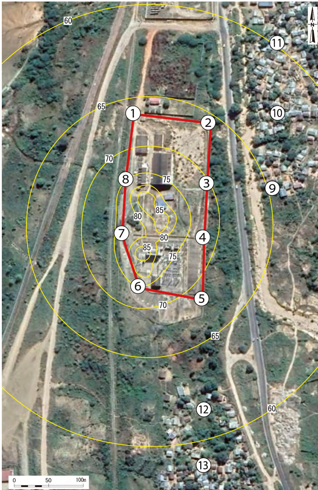
Figure 3-23 Results of Simulating Noise Level (dBA) from Construction Work without Provisional Fence
