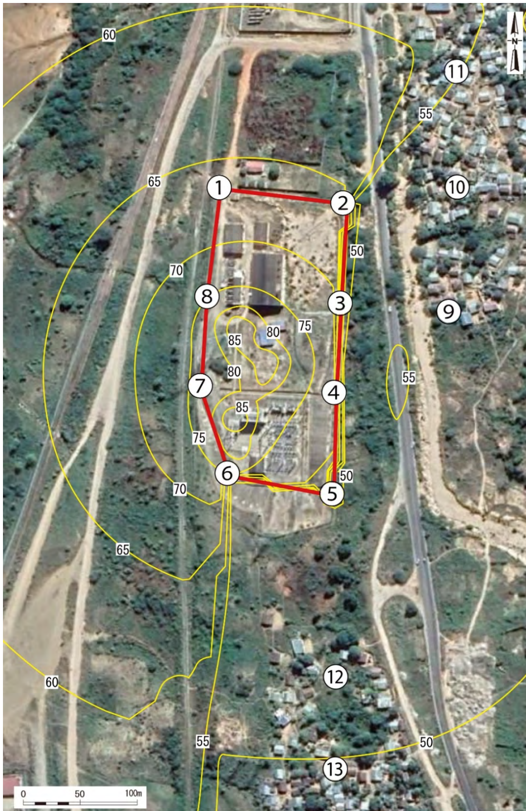
Figure 3-24 Results of Simulating Noise Level (dBA) from Construction Work with Provisional Fence
