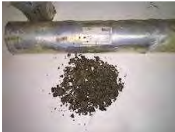
Figure 8. Undisturbed sample of Nampula Central at 5.0m
