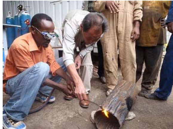
Practice of gas cutting (trainer is directly teaching a trainee)
